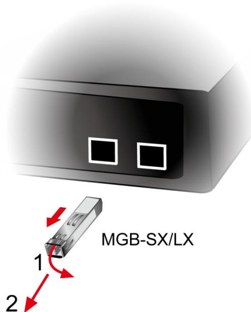
Figure 2-17: How to Pull Out the SFP/SFP+ Transceiver
